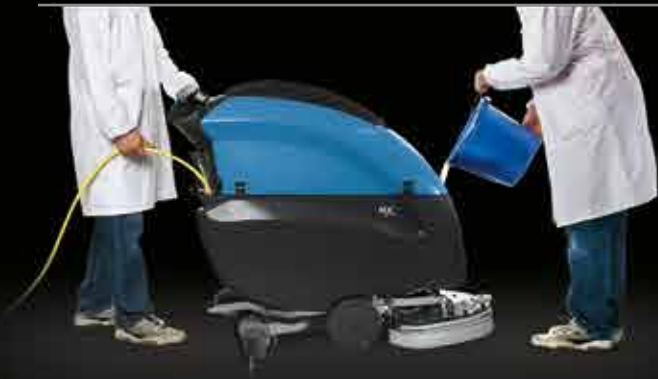
Double water fill opening on the solution tank
