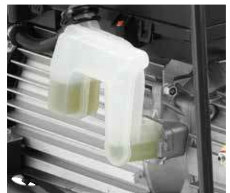
Pump oil tank with oil level sight and fill/empty function.
